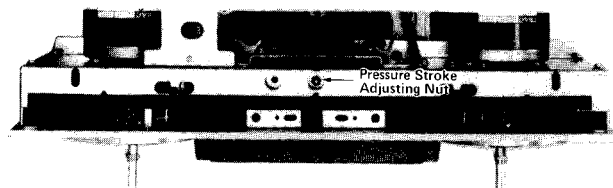
Fig. 2-5 Pinch roller pressure stroke adjustments
