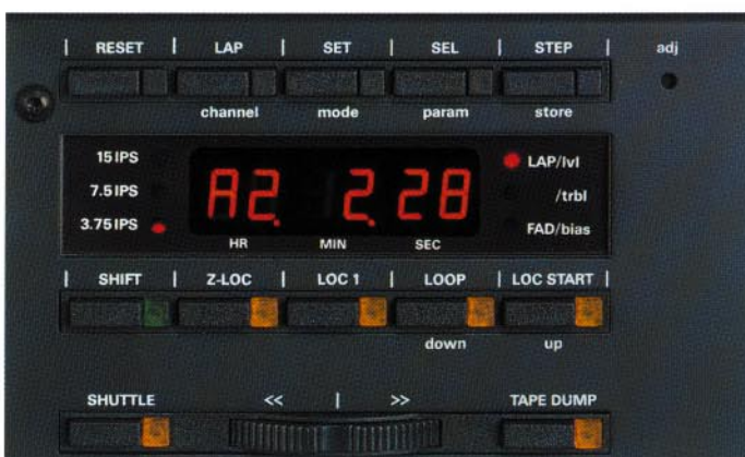
Calibration center: Multifunctional keypad and display for easy audio setup.
