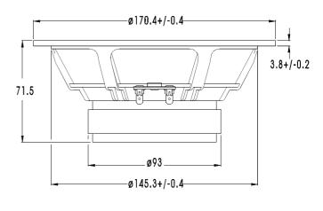
W17E 002 is a 6.5 "Woofer/Midrange unit with an extremely stiff, yet light injection moulded magnesium cone which gives tremendous bass precision and midrange detail.
