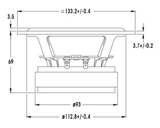
W14CY001 is a 5 " Woofer/Midrange unit with an extremely stiff, yet light injection moulded magnesium cone which gives tremendous bass precision and midrange detail.
