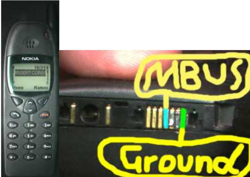
My humble 6110 and its pinout. Soldering wires directly onto the phone does not hurt it if you were wondering. Since people have asked I have put more connection pinouts at the bottom of this page, 8810,3310,3210, 8210, 8250
