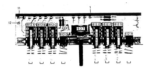
Fig. 14 Printed wiring board with components, Unit 2
