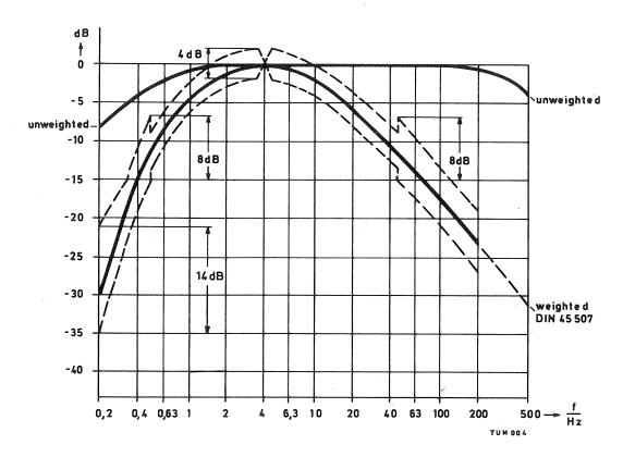
Fig. 7 Transmission characteristic of evaluated and non-evaluated measurements
