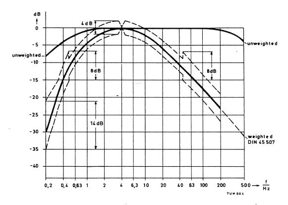
Fig. 7 Transmission characteristic of weighted and unweighted measurement
