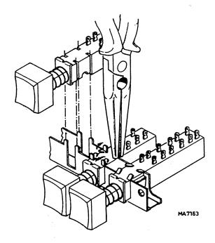
Fig. 8 Replacing a switch of the pushbutton unit
