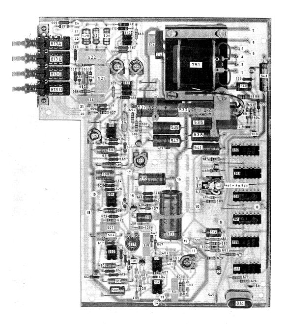
Fig. 13 Printed wiring board with components, Unit 1
