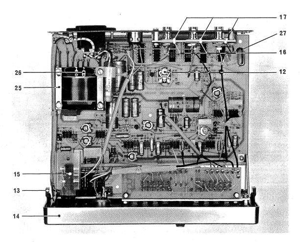
Fig. 12 Inside view bottom side, mechanical parts
